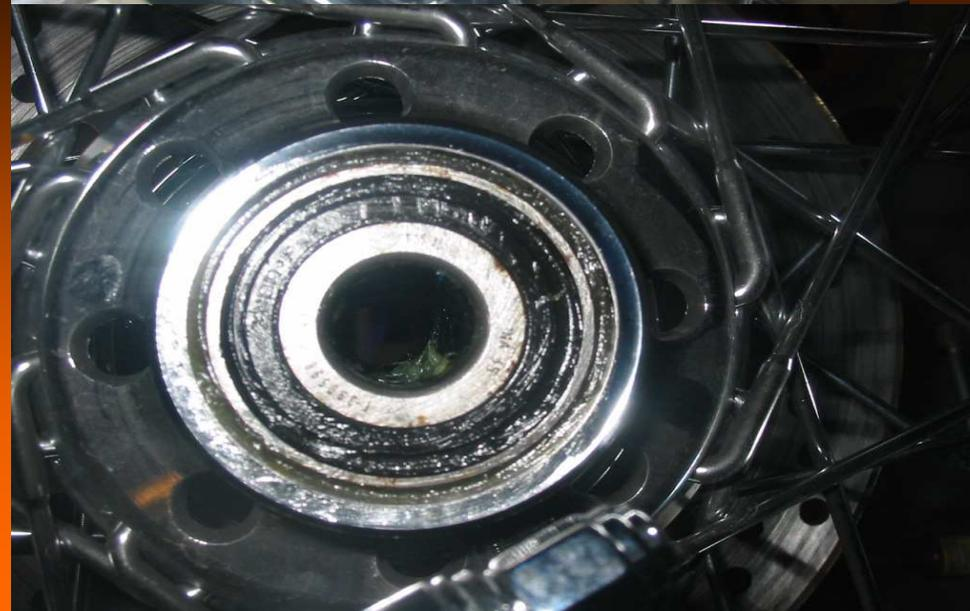
INSERIAMO QUINDI IL PERNO UTILIZZANDO LO STESSO SISTEMA PER LO SMONTAGGIO, CIOE' LO SPESSORE SOTTO LA RUOTA, QUINDI INSERIREMO IN SEQUENZA LA CAMPANA, LA RUOTA E LO SPESSORE IN QUESTO CASO QUELLO NUOVO CROMATO, QUINDI I COPRI PERNO CROMATI. INFINE LA PINZA DEL FRENO.
